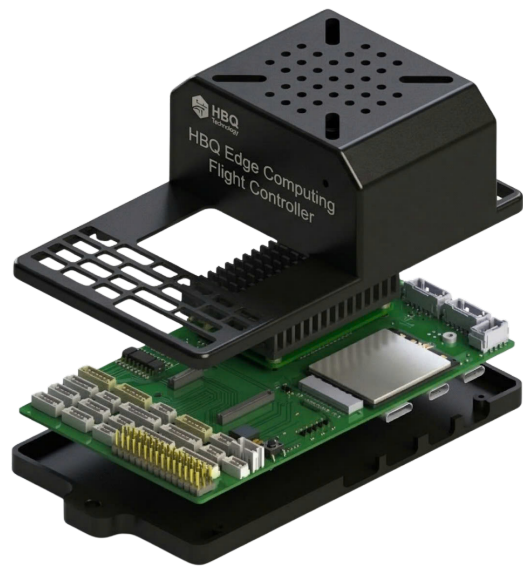
Modular enclosure, compute layer and flight-control baseboard.
